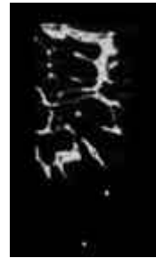
Figure 2: LII Signal from a 5 bar, f = 1.8 Iso-octane-Air Explosion Flame [3, 5] (Flame radius \sim 60 mm)
