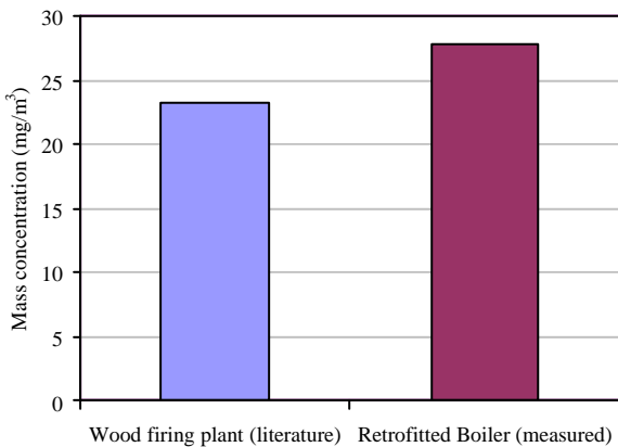
Figure 3 Mass concentration of particles from a wood boiler and retrofitted boiler
