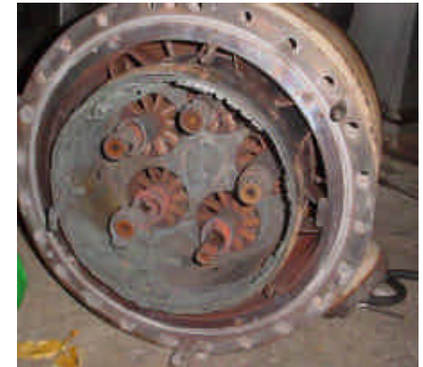
Damage due to high dynamics
